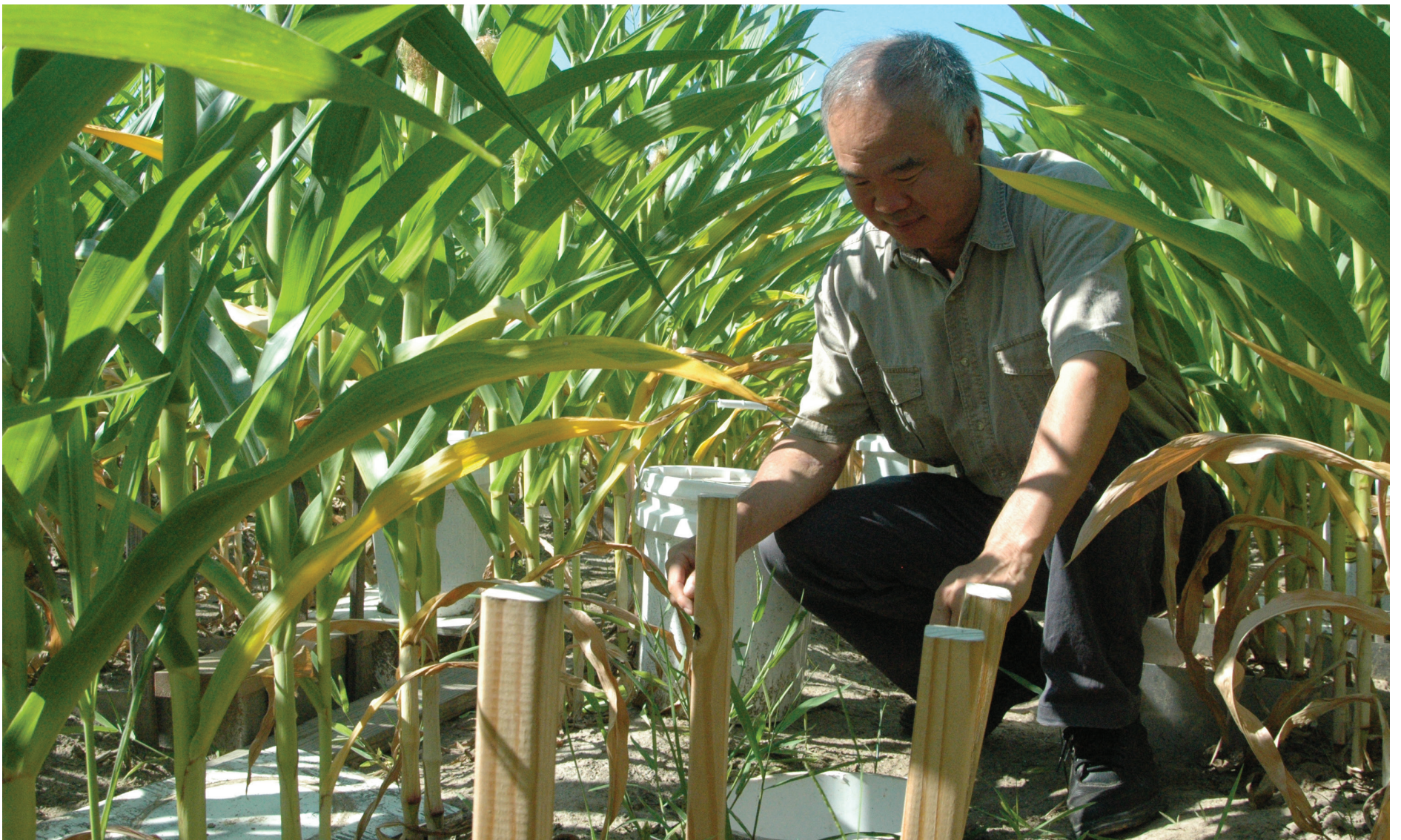
LSU AgCenter soil chemist Jim Wang works with mini-plot water sample collectors, which are used to trace how much nitrogen goes to the plant, soil and water. Photo by Randy LaBauve
